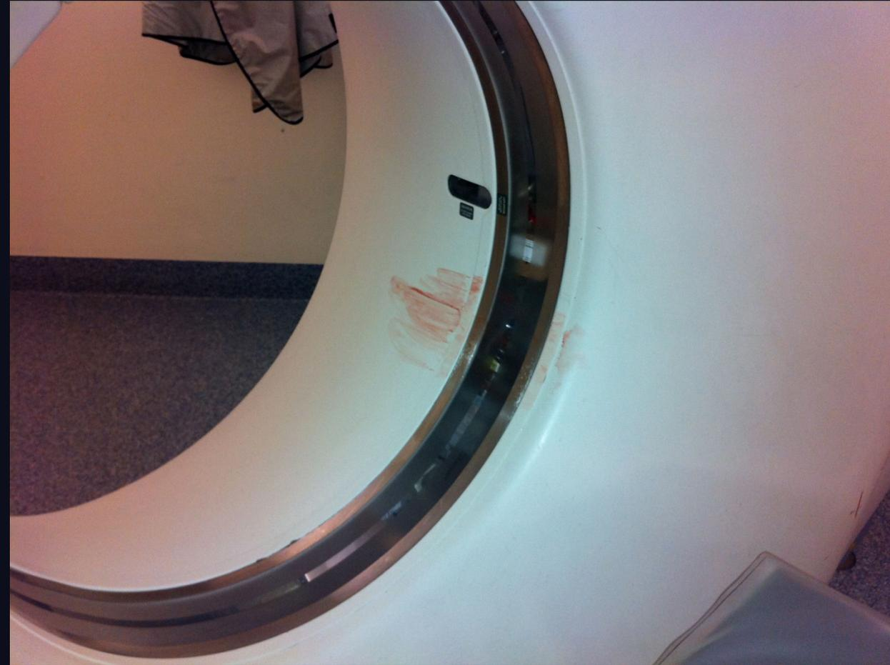
A common problem has existed since the inception of CT with spillage of contrast, blood or bodily fluids on the gantry, which seep through the spaces between the mylar window and gantry surface that leaks on the detectors. These substances cause degradation in image quality, especially if iodinated contrast extravasated from the patient.
