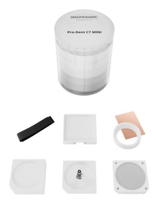
This kit is a versatile set of phantoms and software for carrying out constancy and acceptance tests of Intra-oral, OPG, CBCT, DVT and other 3D imaging devices. Thanks to the Diagnomatic subscription all tests can be quickly and effortlessly automatically analysed online.
