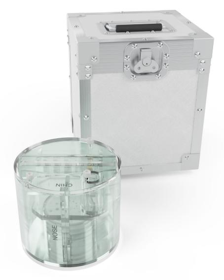
ACR accredited Medium MRI phantom for comprehensive evaluation of critical imaging parameters of magnetic resonance imaging (MRI) in a time efficient manner. The phantom can be used for the measurement of absolute values for calibration purposes. However, its design is optimized for time efficient daily quality assurance too.
