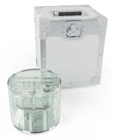
Large MRI phantom for comprehensive evaluation of critical imaging parameters of magnetic resonance imaging (MRI) in a time efficient manner. The phantom can be used for the measurement of absolute values for calibration purposes. However, its design is optimized for time efficient daily quality assurance too.
