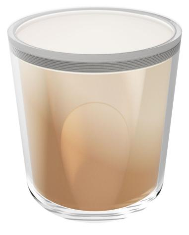
This stability (agar) phantom consists of a cylindrical phantom and agar material inside. Using this phantom a Signal to Noise Ratio, Signal Fluctuation to Noise Ratio, drift, and other imaging measures over a 100-volume or 200-volume fMRI scan can be performed. The agar phantom has characteristics similar to the T2 measures of a human head, but provides no change in signal. The T1 and T2 characteristics of the agar phantom at 3T are ~900 ms T1 and 30 ms T2.
