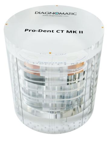
The new Pro-Dent CT mk II phantom is a versatile quality control tool of dental Cone-Beam CT, Dental Volume Tomography (DVT) and other 3D imaging devices according to the Radiation Protection Report no 172 by SEDENTEXCT.
