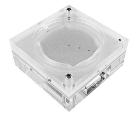
The Pro-Dent DIN 2D is a universal phantom for carrying out constancy and acceptance tests of conventional and digital dental X-ray units (intra-oral, panoramic and cephalometric).
