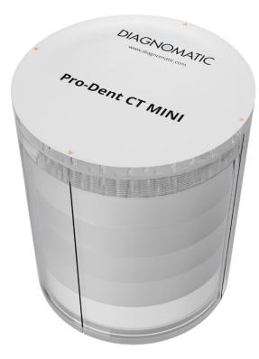
Pro-Dent CT MINI phantom is a versatile quality control tool of dental Cone-Beam CT, Dental Volume Tomography (DVT). and other 3D imaging devices with even the smallest FOV (Field Of View).
