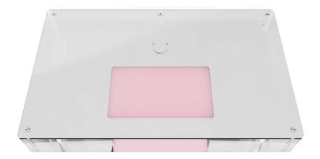
This ACR accredited Full Field phantom was designed to test the performance of a digital mammographic system by evaluating the system's ability to image small structures similar to those found clinically: micro-calcifications, fibrous structures in ducts and tumor-like masses. It is similar to the Pro-MAM Accreditation phantom, the main difference being the size: the FF (Full Field) version is larger and covers the entire image detector, thus eliminating scatter.
