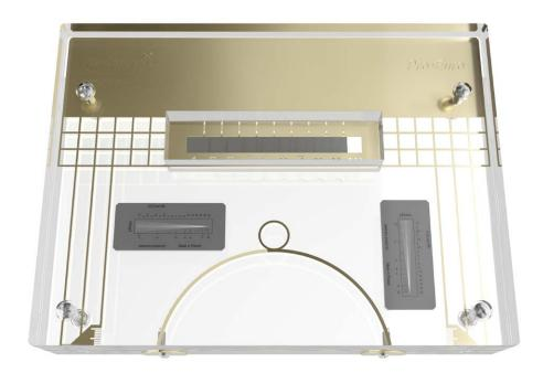
Pro-Euro phantom is used for **monitoring technical parameters** of mammography imaging systems according to the requirements of the "**European Guidelines for Quality Assurance in Mammography Screening**" and IEC 61223-3-2:
