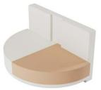
Pro-MAM CESM Phantom is used for Image Quality Evaluation of Contrast-Enhanced Digital Mammography systems. The phantom demonstrates the presence and absence of iodine in tissues by containing different iodine concentrations and non-iodine breast tissue substitutes. The Pro-MAM CESM represents an average human breast in size and shape.
