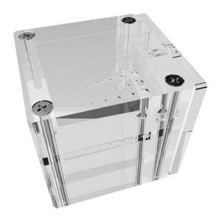
The phantom for **performance testing of mammography** X-ray units. It has **49 holes** that generate subtle changes in contrast. It can be used to **detect small variations** in system's performance.
