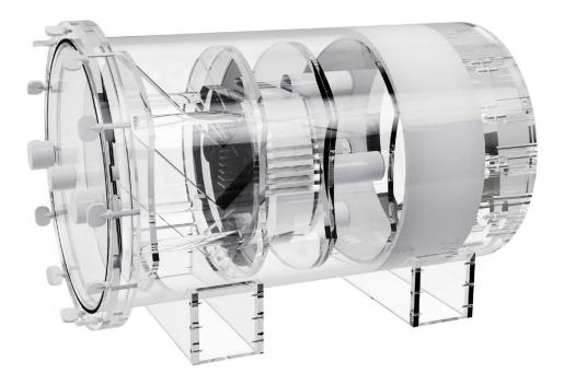
The Pro-CT AAPM phantom can be used for **carrying out tests of computed tomography systems** according to **Report no. 1 of the AAPM** (American Association of Physicists in Medicine).
