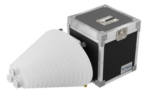
The phantom used for AEC testing on CTs. All mounting and positioning features are the same as in the Pro-CT mk II phantom for off-the-table measurement.
