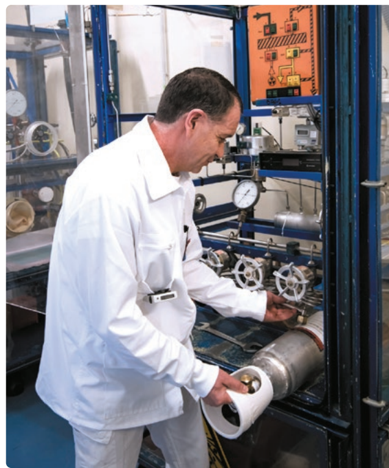
© LEA Installation of an empty ^{85}\text{Kr} cylinder
