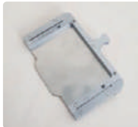
Drawer in closed position. Position adopted during normal operation of the atmospheric contamination monitor. The tray is retracted, shielding against the flow of alpha particles generated by the source.
