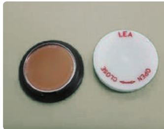
1.6 in (40 mm) active diameter source deposited in 1.9 in (47 mm) diameter customer planchet.
