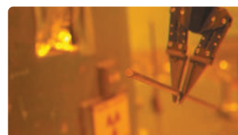
© IRSN Saclay Remote handling of sources of gamma radiation used to study materials' behavior under irradiation.
