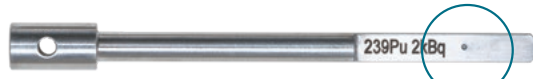
Example of needle support on which radionuclides are deposited : rod diameter 0.2 x 3,1 in (5 x 80 mm) long.
