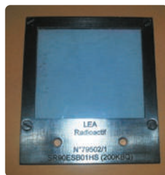
Active size source 1.5 x 1.7 in, external dimension 1.7 x 1.9 in mounted on a specific stainless steel support
