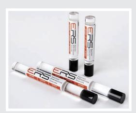
ERS offers a wide range of rod sources that are used for calibrating well counters and thyroid uptake systems. Rod sources are constructed of acrylic material and have a flat base which allows easy positioning in the vertical position required for consistent accuracy of the calibration process.
