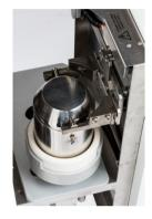
Uncapping of the lead pot and perforation of the multi dose vial septum are performed automatically, as well as the dose drawing from the vial, within the fully shielded compartment for a full operator protection throughout the whole process. A specific study performed with an innovative dose rate monitor (Aegis ED3) proved a significant decrease of the staff doses using KARL100.
