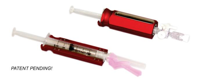
The sliding syringe shielding is designed with a tungsten shielding of 2,5 mm. and a lead glass window with a density of 5,2 g / cm2.
