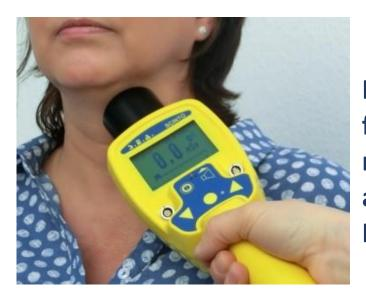
NUVIA's SCINTO is also successfully used to calculate the thyroid dose in emergency centers after a nuclear accident.
